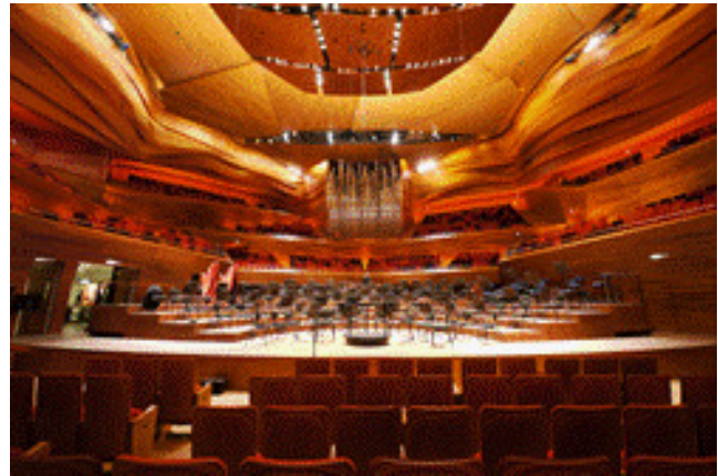
Figure 2: Suspended Acoustic Canopy and Orchestra Risers on Stage
